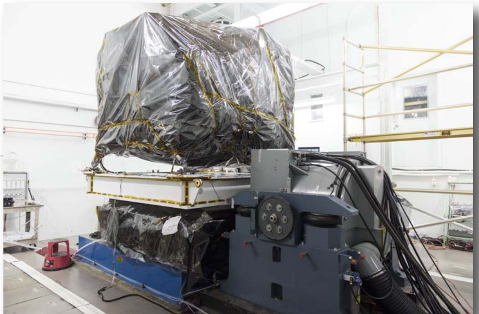
Figure 2: The ISIM prime module (the ISIM structure plus the science instruments) on the vibration table for sinusoidal sweep testing. As the vibration facility is not a clean room, the ISIM is carefully bagged and purged for contamination control.
