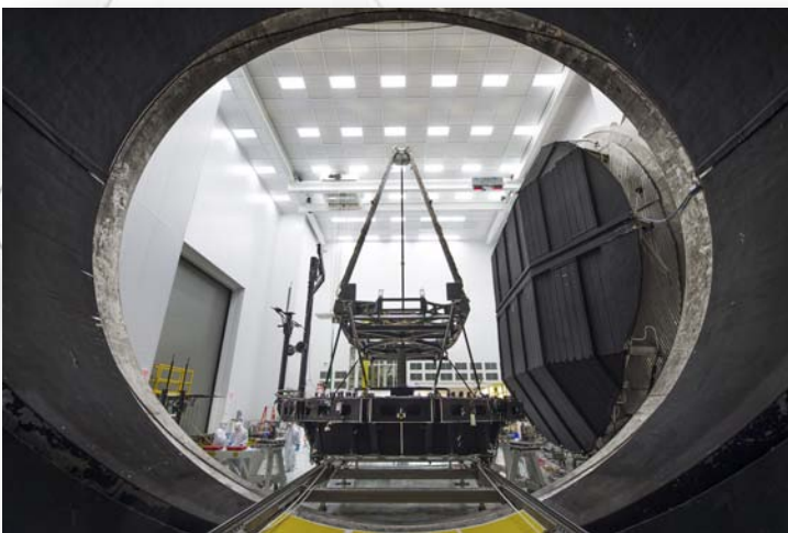
JWST's pathfinder backplane outside Chamber A at NASA Johnson. Credit: NASA/Chris Gunn
